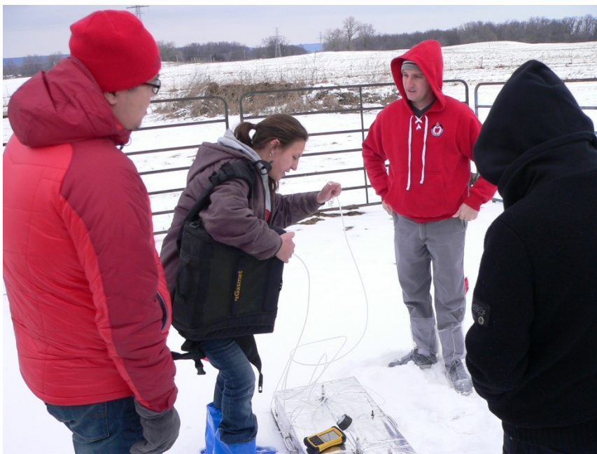
Fig. 1 Associate research specialist Ali Pelletier uses a Fourier transform infrared spectroscopy (FTIR) to measure greenhouse gas fluxes within a stainless steel chamber at the USDA Dairy Forage Research Center on a snowy day in Prairie du Sac, Wisconsin as Dr. Matias Aguerre (red hood) and Fei Sun (red hat) look on. Dr. Aguerre, formerly a post-doctoral research associate with Dr. Michel Wattiaux, is now an Assistant Professor of Animal and Veterinary Science at Clemson University. Photo: Carolyn Betz
