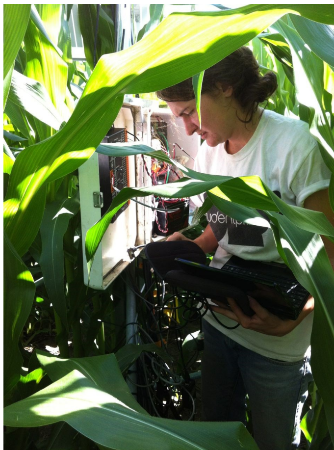
Figure 8. In her research on soil water dynamics, UW-Madison student Elizabeth McNamee (Bland Lab) collects continuous soil water content and matric potential data over the growing season using moisture probes and tensiometers. Preliminary results show little difference among dairy cropping systems in the wet end of the soil water characteristic curve.
