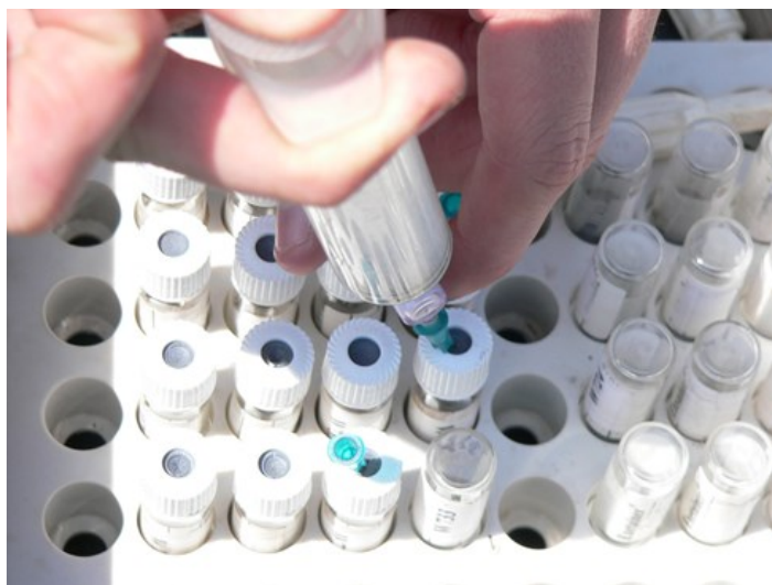
Figure 7. Gases from the chambers are inserted into vials where they are later analyzed for N 2 O, CH 4 and CO 2 . GHG flux curves are then calculated. Photo: Carolyn Betz
