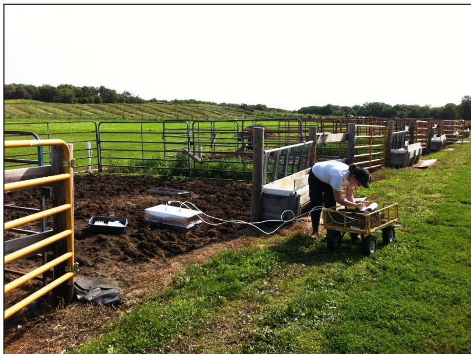
Figure 5. Claire Campbell set up the Fourier transform infrared spectroscopy (FTIR) in the field. Part of her research was to investigate the comparability of data generated through the differing approaches of gas chromatography (GC) versus the FTIR to see if the data generated produced comparable results both in measurement of absolute gas concentration above the soil as well as rate of flux from the soil. This is of particular relevance where large databases – such as those used in crop production and climate modeling – will be populated by multiple data streams possibly derived through varying techniques. Both methods measured CO 2 , N 2 O, and CH 4 emissions from soil. Results of 130 paired sampling instances indicate that no significant differences exist between the two techniques in measured CO 2 concentrations, while slight differences were detected in both CH 4 and N 2 O concentrations
