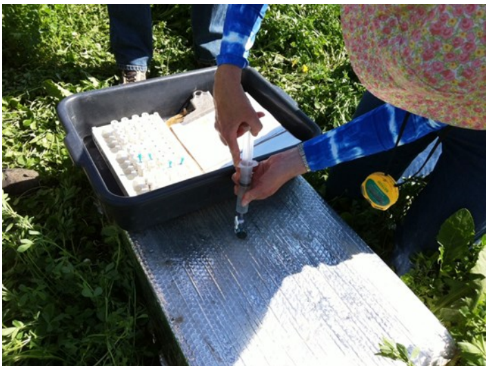
Figure 6. Under the supervision of Dr. Sarah Collier, a technician withdraws gases from a stainless steel greenhouse gas chamber at Arlington Research Station in Wisconsin. Photo: Sarah Collier
